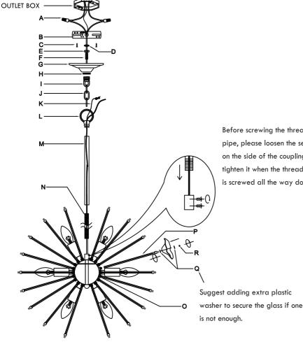
Before screwing the threaded pipe, please loosen the set screws on the side of the coupling, tighten it when the threaded pipe is screwed all the way down.
